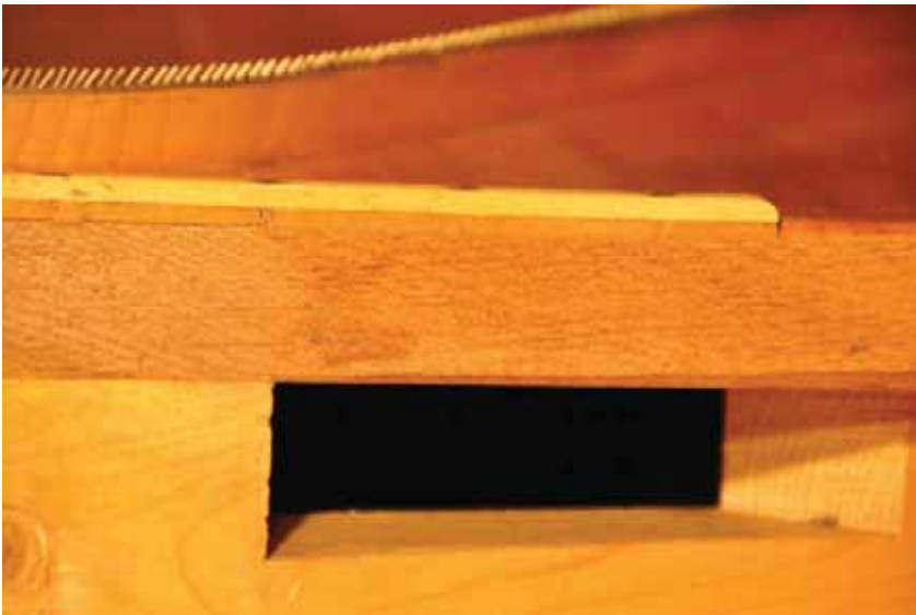
The mouse hole cut opening under the soundboard, with the thickness of the soundboard showing.
