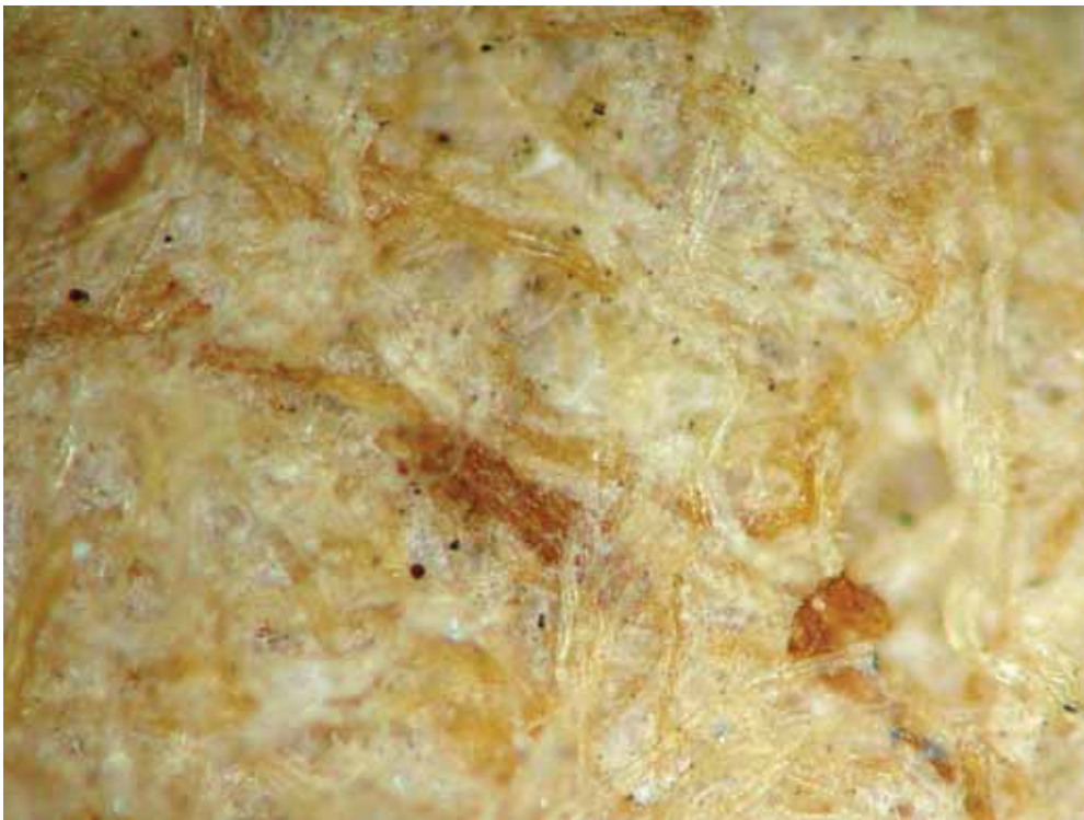
Uncoated side, 100X, epi-illumination - dark field
