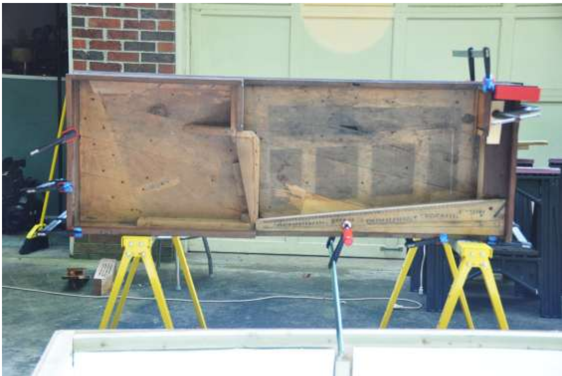
Showing the tothing plane marks for a good glue joint. Original 18 th C marks.
