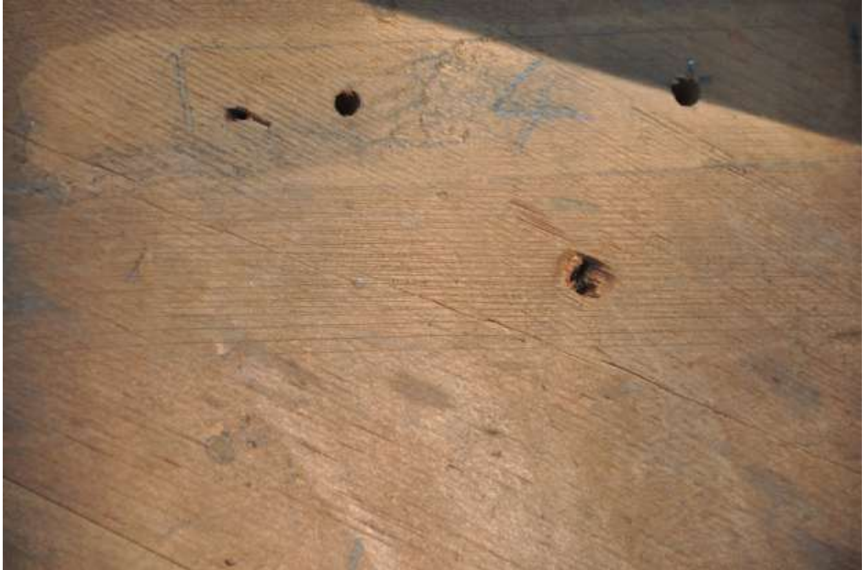
Showing the tothing plane marks for a good glue joint. Original 18 th C marks.
