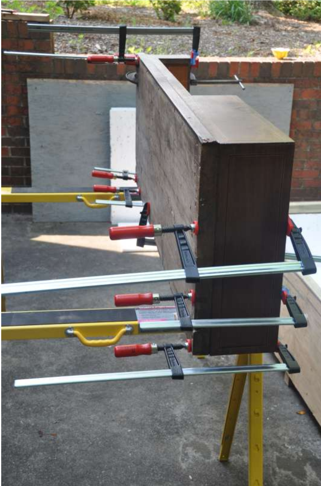
Gluing up the case where it had separated from the bottom due to water logging.
