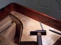
Before working on the hitchpin block the instrument was detensioned and the strings slipped off the hitch pins. As I did not wish to remove the tuning pins I arranged the strings in sets with wires run through the hitch eyes in order and coiled up out of the way but with as little kinking as possible.
