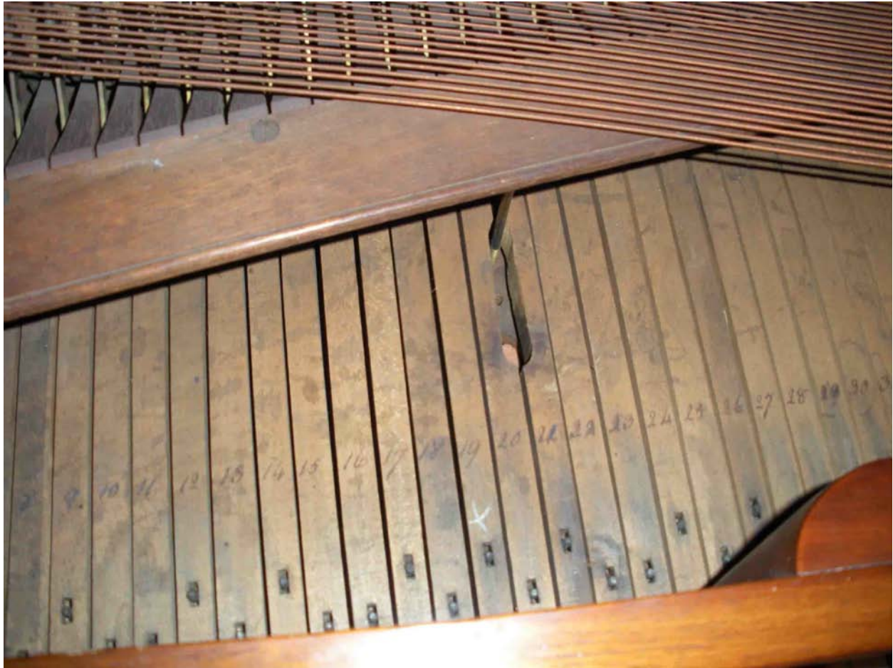
Opening for damper lift actuator.
