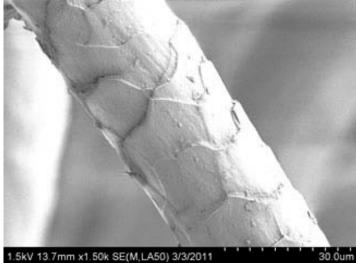
New wool at 250 and 1500X. Note that shaft scale pattern remains similar; both shafts are  $\sim$ 30 microns diameter.
