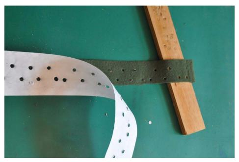
The cloth can now be fitted over the pins and the ends trimmed. These over-the-pin cloths usually were not glued down, but you can secure the ends if desired.
