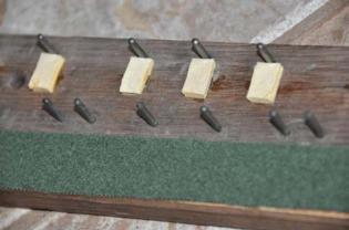
Broadwood used flatter key bottoms and so used a toothed profile cloth for the key balance rail, made as shown below. You can find cuts in the frame from the original installation, so obviously the balance rail cloth was installed full width and rebates cut afterward.
