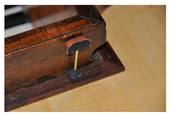
Depressing the pedal pulls down the cross arm, and pushes up on a brass rod, covered in this case in a shoe of sole leather, with a little leather collar to limit the return travel. This impinges only on the lid flap, where a rebate around the edge is covered in close spun flannel. This allows the lid flap to close quietly during performance, and the resulting dynamic control is notable and effective, if difficult to use in modern music interpretation.
