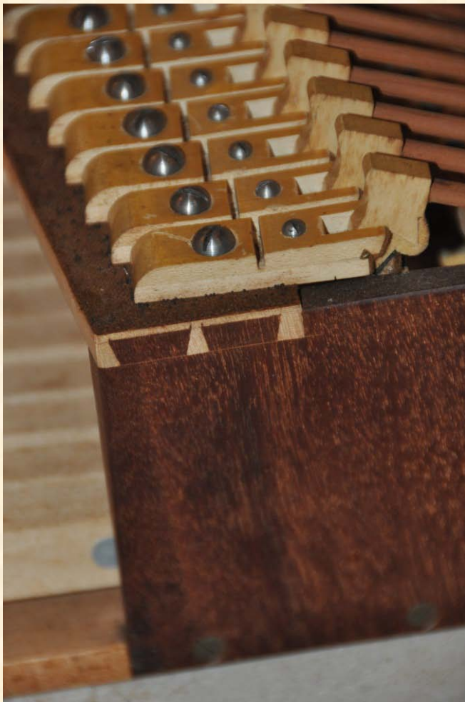
Action frame showing dovetailing
