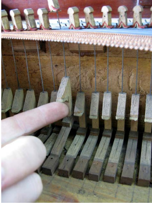
Jacob Ball square with alternate approach to damper levers. These are modified double action jacks, and may have used a spring assist, now missing.
