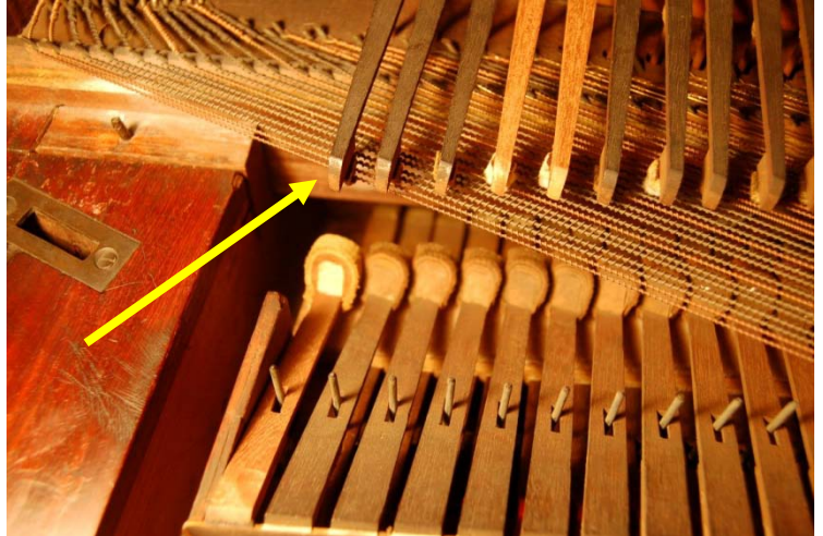
Earlier lever dampers with whalebone springs in rear
