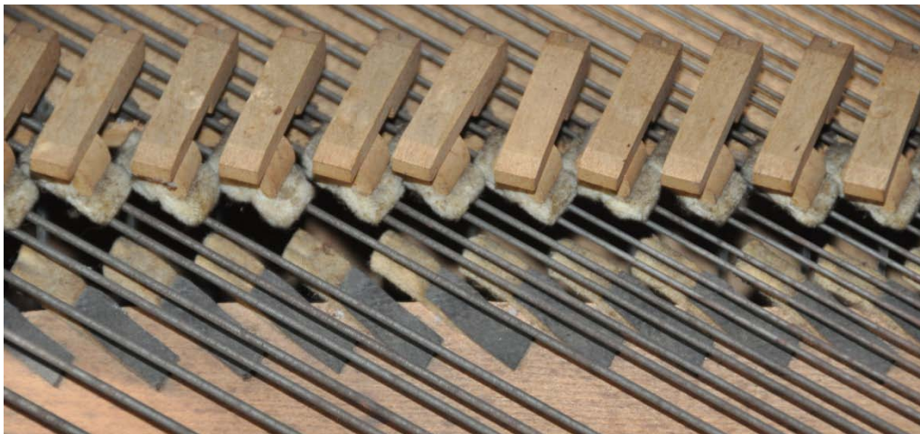
Southwell styled dampers in an 1854 Newman & Brother piano of Baltimore.
