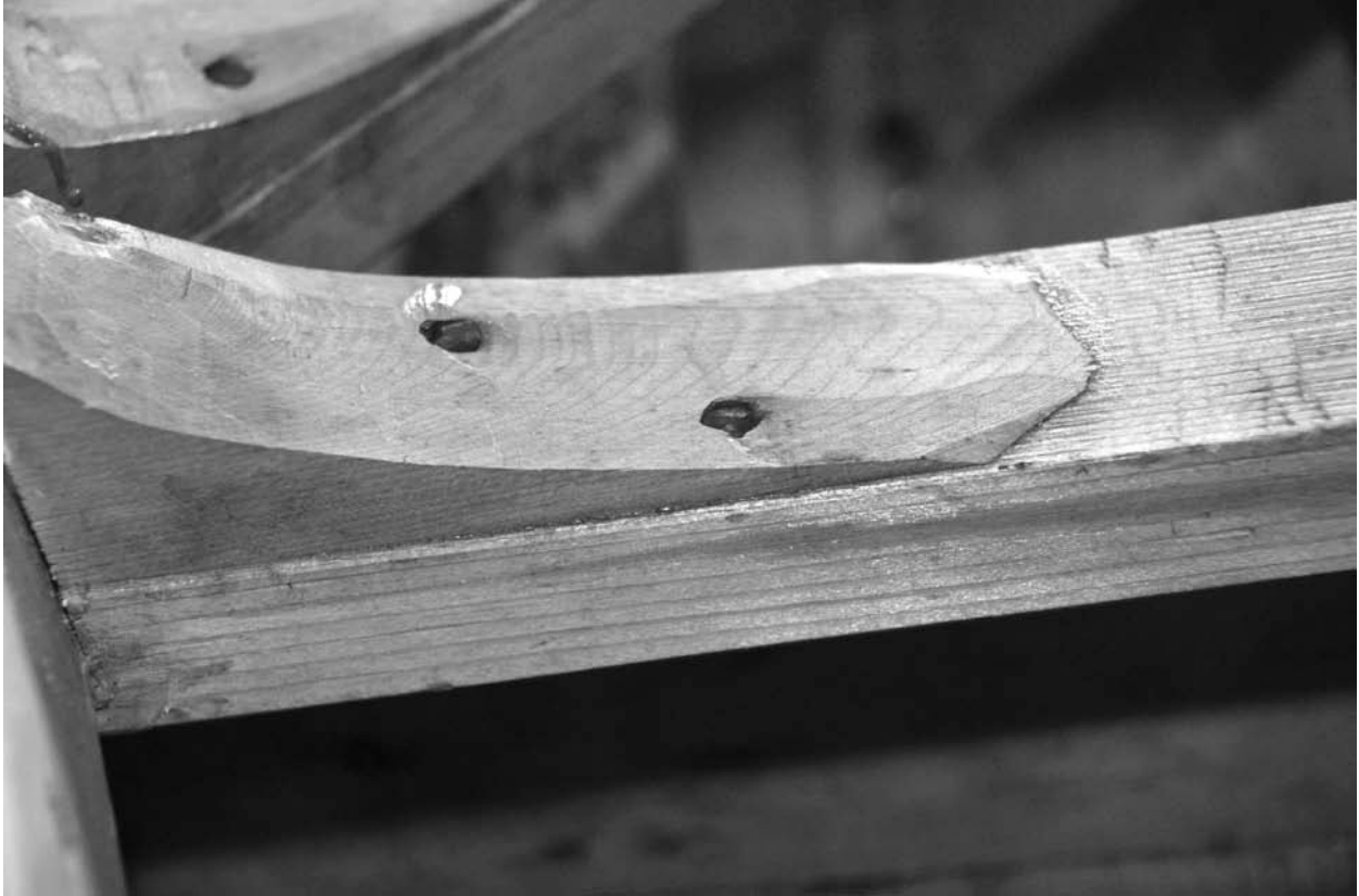
Figure 11, carved knee at liner bracing showing marks from knife at far right
