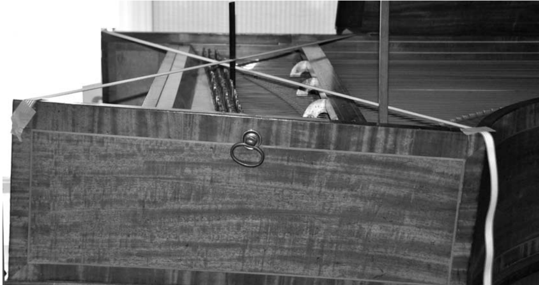
Figure 2, Cheek warp and crossed ribbons to determine extent of displacement.
